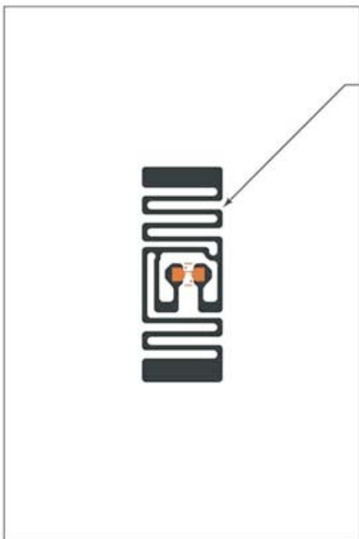
RFID Chip-Inlay Contains the RFID code only.
